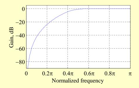
• The lowpass-to-highpass transformation can also be used to transform a highpass filter with a cutoff at  $\omega_c$  to a lowpass filter with a cutoff at  $\hat{\omega}_c$
