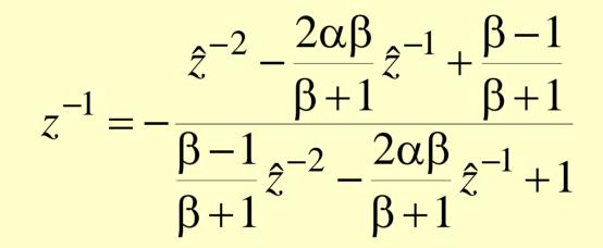
• The parameters  $\alpha$  and  $\beta$  are given by  $\alpha = \frac{\cos((\hat{\omega}_{c2} + \hat{\omega}_{c1})/2)}{\cos((\hat{\omega}_{c2} - \hat{\omega}_{c1})/2)}$   $\beta = \cot((\hat{\omega}_{c2} - \hat{\omega}_{c1})/2)\tan(\omega_c/2)$
