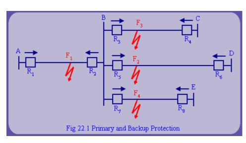
The primary protection should be fast and hence preferably it should be done without anv intentional time delay, while back up protection should operate if and only if corresponding primary relay fails. In fig 22.1, R1 backs operation of relays R<sub>3</sub>, R<sub>5</sub> and R<sub>7</sub>. Typically, distance relays are provided with multiple zones of protection to meet the stringent selectivity and sensitivity requirements. At least three zones of protection are provided for distance relays.
