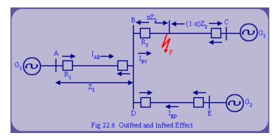
Due to the configuration of generators and loads, we see that  $\vec{I}_{BF} = \vec{I}_{AB} + \vec{I}_{FD}$
