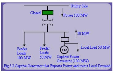
Consider a medium voltage distribution system having local generation (e.g., captive power generation) as shown in fig 3.2 which is also synchronized with the grid. During grid disturbance, if plant generators are not successfully isolated from the grid, they also sink with the grid, resulting in significant loss in production and damage to process equipments. The following relays are used to detect such disturbances, its severity and isolate the inplant system from the grid.
