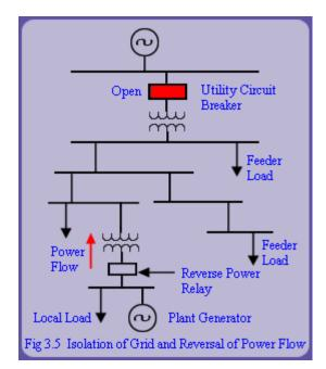
Distribution systems are radial in nature. This holds true for both utility and plant distribution systems. If there is a fault on the utility's distribution system, it may trip a breaker thereby isolating plant from the grid. This plant may still remain connected with downstream loads as shown in fig 3.4 and 3.5. Consequently, power will flow from the plant generator to these loads.
