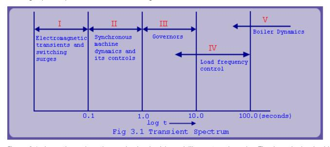
Figure 3.1 shows the various time scales involved in modelling system dynamics. The dynamics involved in switching, lightening, load rejection etc have a high frequency component which die down quickly. In analysis of such dynamics, differential equations associated with inductances and capacitances of transmission lines have to be modelled. Such analysis is restricted to a few cycles. It is done by Electromagnetic Transient Program (EMTP).
