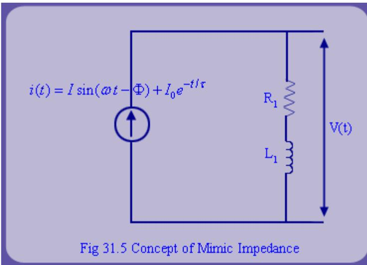
Mimic impedance is an impedance whose  $X/R$  ratio is identical to the  $X/R$  ratio of transmission lines. In that sense, it mimics a transmission line.
