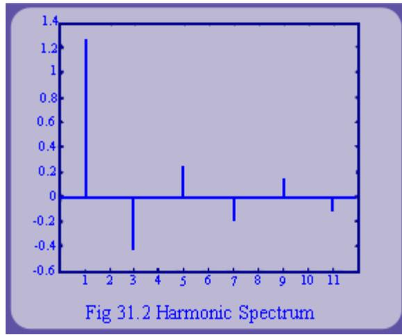
This signal is sampled at a rate of 10 samples per cycle and full cycle Fourier method is applied to estimate the fundamental. In addition noise is introduced using random number generator. The true value of fundamental component is  $\frac{4}{\pi} \times 10 = 12.7324$ .
