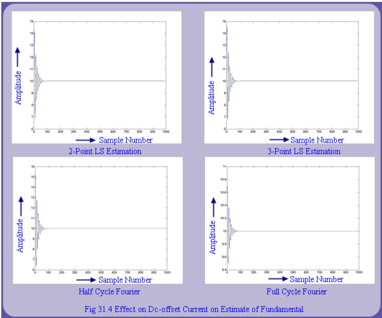
Fig 31.4 Effect on Dc-offset Current on Estimate of Fundamental
