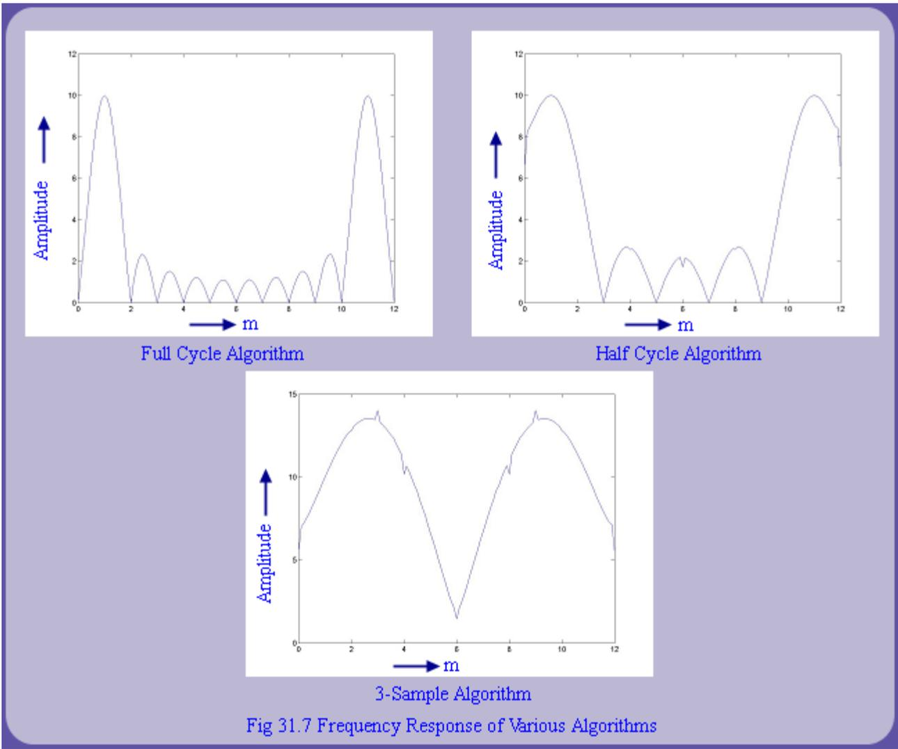
Fig 31.7 Frequency Response of Various Algorithms
