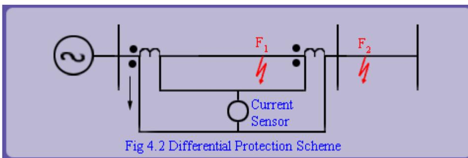
However with a differential protection the CT location provides 'crisp' demarcation of zone of protection of CT (see fig 4.2). The fault  $F_1$  is in the relay's zone of protection, but fault  $F_2$  is not in its jurisdiction. Because differential protection scheme do not require time discrimination to improve selectivity, they are essentially fast. These aspects will be discussed in more detail in the later lectures.
