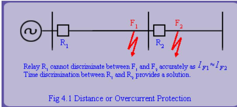
Like sensitivity, selectivity also implies an ability to discriminate. A relay should not confuse some peculiarities of an apparatus with a fault. For example, transformer when energized can draw up to 20 times rated current (inrush current) which can confuse, both overcurrent and transformer differential protection. Typically, inrush currents are characterized by large second harmonic content.
