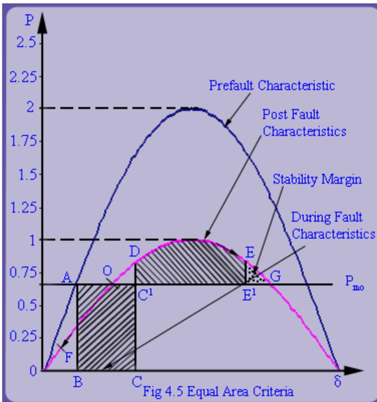
At point E,  $\Delta\omega = \omega - \omega_0$  is equal to zero and the extreme point of swing is reached. As  $P_e > P_m$ , the deceleration continues and hence the rotor starts retarding. At point O,  $P_e = P_m$  the acceleration is zero, but machine speed is lower than nominal speed  $\omega_0$  ( $2\pi f_0$ ). Consequently, the angle  $\delta$  continues to fall back.
