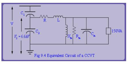
inductor has an inductance of 497H and resistance of 4620  $_{\Omega}$ . X<sub>m</sub> of the VT referred to 6.6 kV side is 1M  $_{\Omega}$ , core loss = 20 watts per phase, VA burden = 150VA per phase. Value of C<sub>m</sub> for compensating the current drawn by X<sub>m</sub> is equal to  $3.183 \times 10^{-9} F$ .
