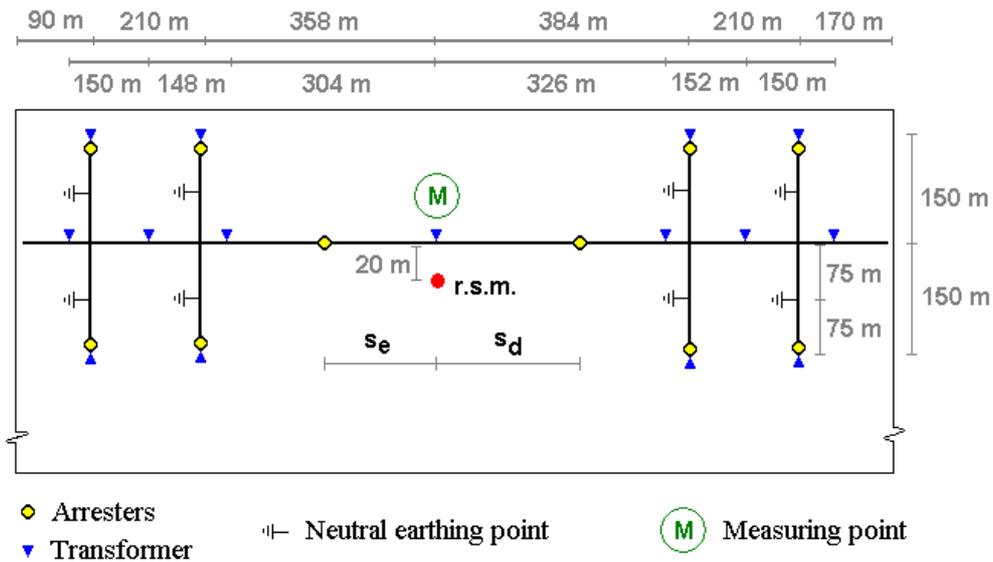
Fig. 14 – Test configuration related to the voltage waveforms presented in Figure 13. Neutral conductor grounded at the middle of each lateral and at all installation points of transformers and surge arresters; r.s.m.: stroke location.
