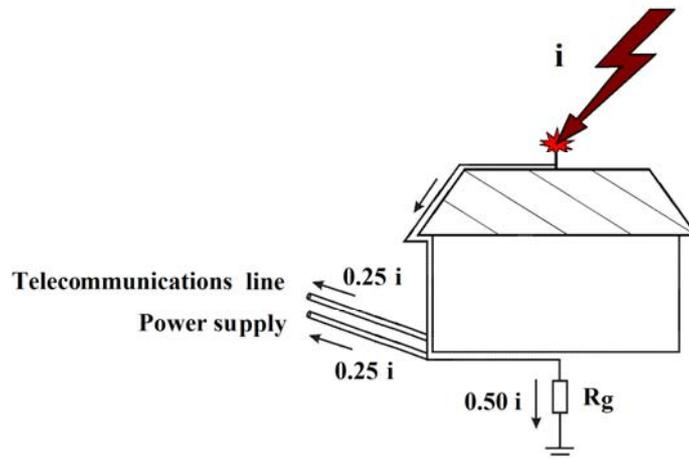
Fig. 17 - Injection of surges into the low-voltage power line due to a direct strike to an end-user installation.
