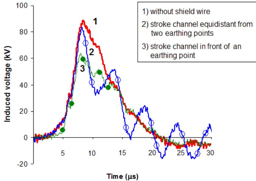
Fig. 9 – Induced voltages (phase-to-ground) - influence of the relative position of the stroke channel with respect to the earthing points (adapted from [5]). Lightning current: amplitude 24.9 kA, equivalent front time 3.5  $\mu$ s; stroke location at a distance of 70 m from the distribution line;  $x_g = 750$  m;  $R_g = 0 \Omega$ ; height of the shield wire: 9 m; perfectly conducting earth.
