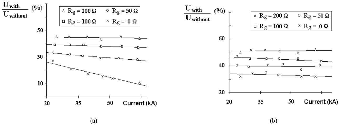
Fig. 15 - Ratio of the voltages induced on lines with and without MO surge arresters ( $U_{with}/U_{without}$ ) as a function of the stroke current magnitude (adapted from [9]). Stroke location is 70 m from the lines;  $tf = 3.2 \mu s$ ; arrester spacing = 300 m.
