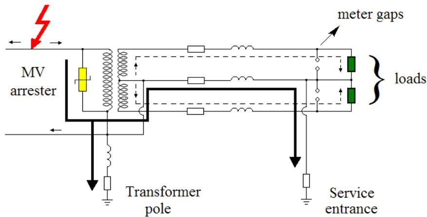
Fig. 21 - Injection of current into the neutral due to a direct strike to the MV line.
