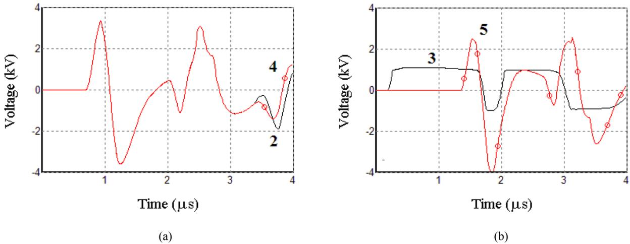
Fig. 26 - Phase-to-neutral induced voltages at points 2, 3, 4, and 5 of Figure 23 considering a subsequent stroke current with amplitude  $I = 29.2$  kA. Configuration 2 (arresters only at the transformer terminals).
