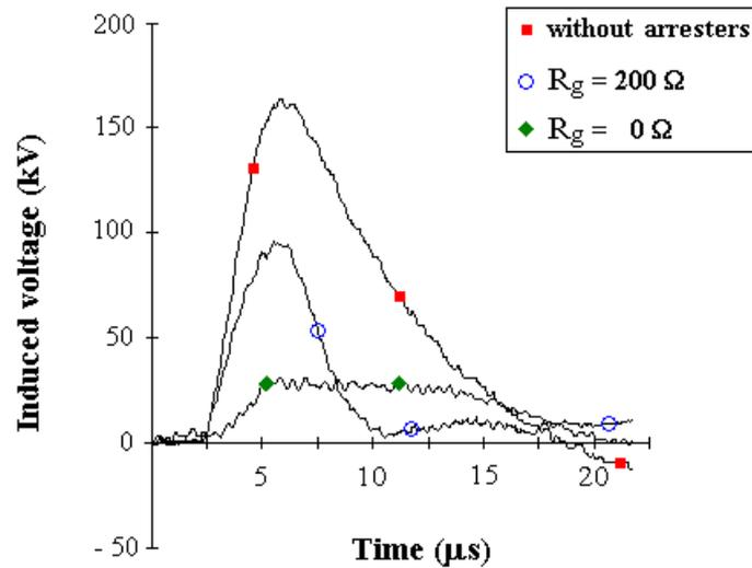
Fig. 16 - Voltages induced on lines with and without surge arresters. Lightning strike point is in front of a set of arresters, at a distance of 70 m from the line (adapted from [9]).  $I = 38 \text{ kA}$ ;  $tf = 3.2 \mu s$ ; arrester spacing = 600 m.
