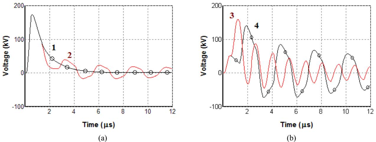
Fig. 10 – Induced voltages by a subsequent stroke of 24 kA at the point closest to the lightning channel.
