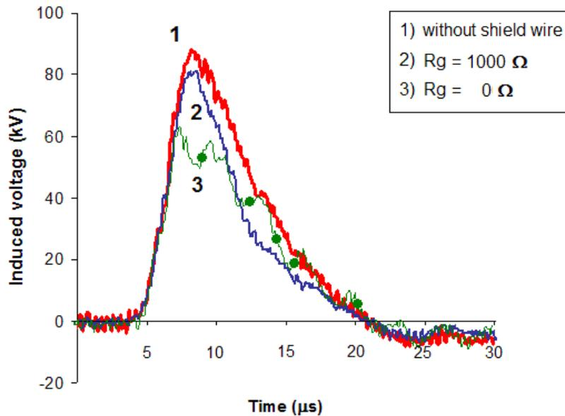
Fig. 8 – Induced voltages (phase-to-earth) at the point closest to the stroke location – influence of the earth resistance (adapted from [5]). Lightning current: amplitude 24.9 kA, equivalent front time 3.5  $\mu$ s; stroke location equidistant from two earthing points, at a distance of 70 m from the distribution line; distance of 450 m between adjacent earthing points; height of the shield wire: 9 m; perfectly conducting earth.
