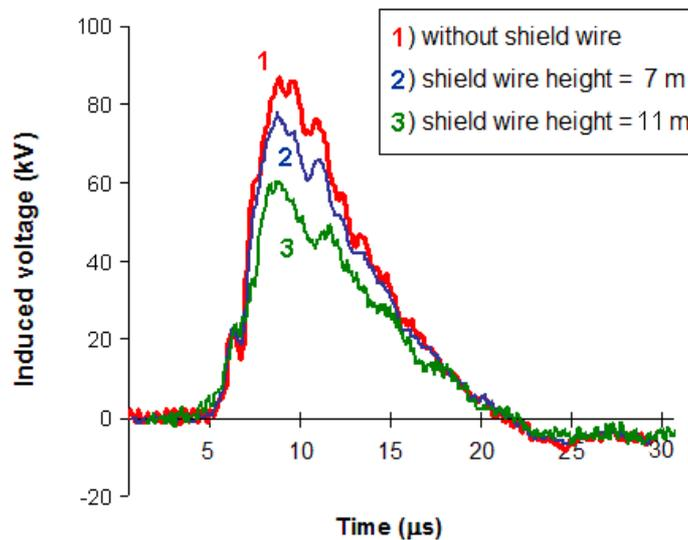
Fig. 7 – Induced voltages (phase-to-earth) at the point closest to the stroke location – influence of the height of the shield wire (adapted from [5]). Lightning current: amplitude 24.9 kA, equivalent front time  $3.5\ \mu\text{s}$ ; stroke location in front of an earthing point, at a distance of 70 m from the distribution line; earthing spacing: 450 m; earth resistance:  $50\ \Omega$ ; perfectly conducting earth.
