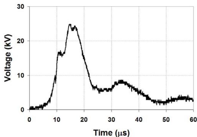
Fig. 6 – Example of a typical lightning induced voltage.
