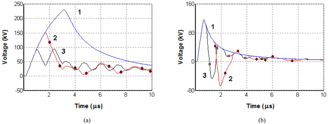
Fig. 12 – Induced voltages at the point closest to the lightning channel.- influence of the distance between adjacent surge arresters.
