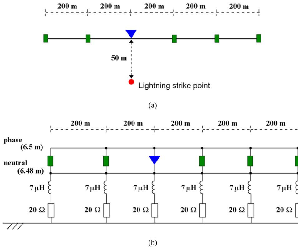
Fig. 20 - Low-voltage line configuration considered in the simulations presented in Figure 19. The triangles and the rectangles denote, respectively, the distribution transformer and the low-voltage power installations.
