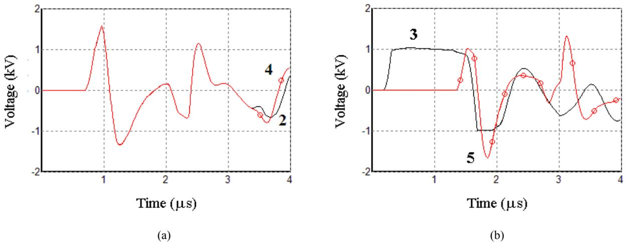
Fig. 25 - Phase-to-neutral induced voltages at points 2, 3, 4, and 5 of Figure 23 considering a typical subsequent stroke current ( $I = 12$  kA). Configuration 2 (arresters only at the transformer terminals).
