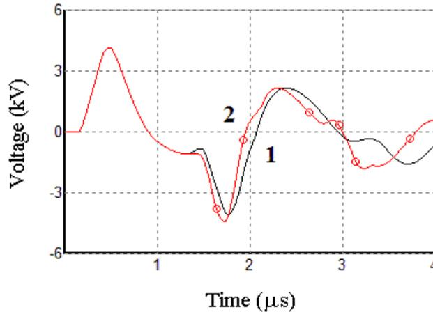
Fig. 24 - Phase-to-neutral induced voltages at Point 4 of Figure 23 when the stroke location is in front of it, at a distance of 50 m.  $I = 12$  kA. Curve 1: configuration 1; curve 2: configuration 2.
