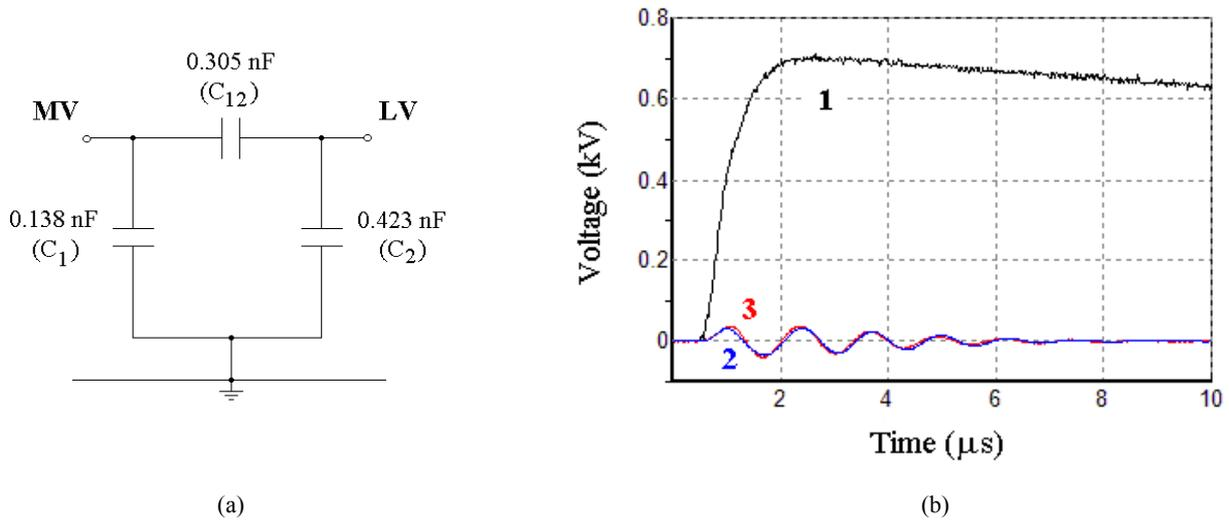
Fig. 18 - Equivalent capacitive PI-circuit and comparison of measured and calculated phase-to-neutral voltages transferred to the secondary of a 30 kVA distribution transformer, in the no-load condition, for a standard 1.2/50  $\mu\text{s}$  impulse voltage of 1.7 kV applied to the primary terminals short-circuited.
