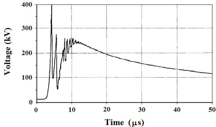
Fig. 1 – Example of a typical overvoltage due to a direct strike to the MV line (adapted from [16]).
