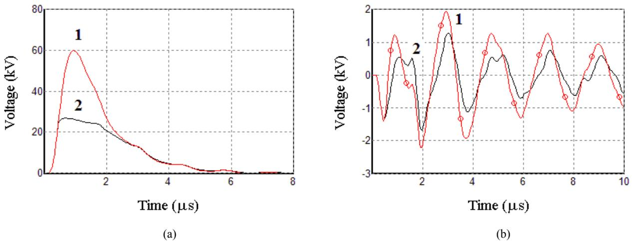
Fig. 19 - Phase-to-neutral voltages at the transformer terminals considering a typical subsequent stroke current of 12 kA. Stroke location in front of the transformer, at a distance of 50 m from the LV line (configuration depicted in Figure 20).
