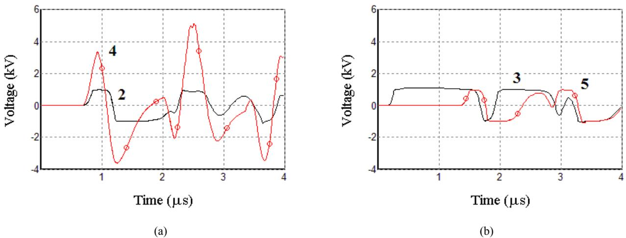
Fig. 27 - Phase-to-neutral induced voltages at points 2, 3, 4, and 5 of Figure 23 considering a subsequent stroke current with amplitude  $I = 29.2$  kA. Configuration 3 (arresters at points 1, 2, 3, 5, and 6).
