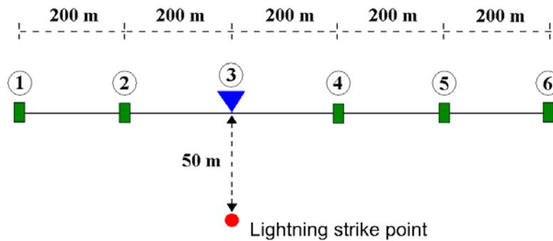
Fig. 23 - Low-voltage line configurations. The triangle and the rectangles denote, respectively, the distribution transformer and the low-voltage power installations. Configuration 1: line without arresters; configuration 2: arresters only at Point 3; configuration 3: arresters at points 1, 2, 3, 5, and 6.
