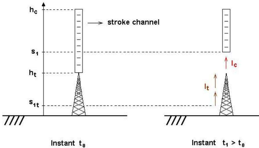
Fig. 2 - Lightning strike to an elevated object.  $h_t$ : height of the strike object;  $h_c$ : height of the upper extremity of the stroke channel;  $I_c$  and  $I_t$ : currents in the stroke channel and in the strike object, respectively;  $s_1$  and  $s_{1t}$ : heights, at instant  $t_1$ , of the current front in the channel and in the strike object, respectively (adapted from [56]).
