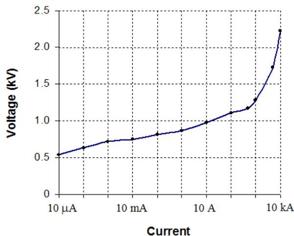
Fig. 22 - V/I characteristic of the secondary MOV arresters.
