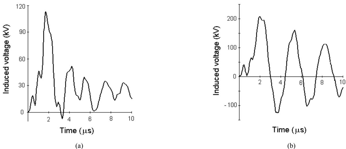
Fig. 13 - Measured phase-to-earth induced voltages considering different distances between surge arresters and measuring point.
