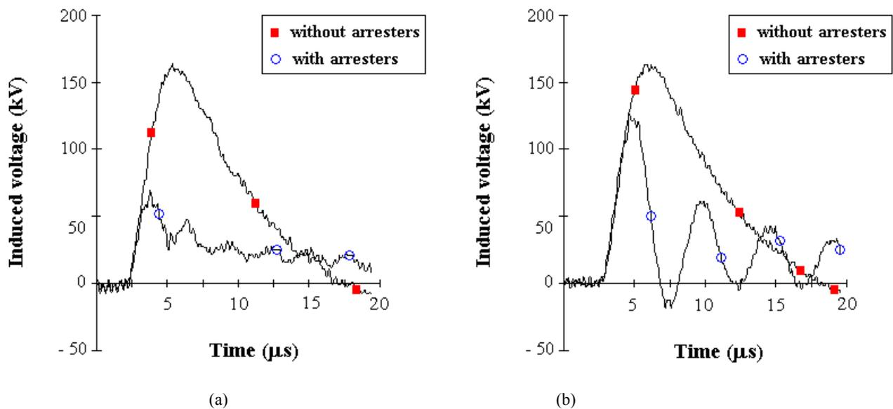
Fig. 11 - Voltages induced on lines with and without surge arresters (s.a.), at the point closest to the stroke location, for arrester spacings of 300 m and 600 m. Lightning strike point 70 m from the line and equidistant from two sets of arresters (adapted from [9]).  $I = 38$  kA;  $t_f = 3.2$   $\mu$ s;  $R_g = 50$   $\Omega$ .
