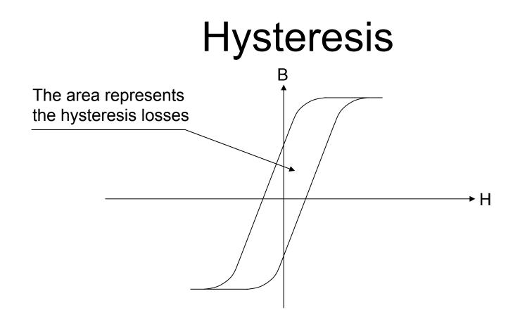
Hysteresis is caused by internal friction in the material. The magnetic domain wall movement, causing the magnetic flux density to lag the magnetic field
