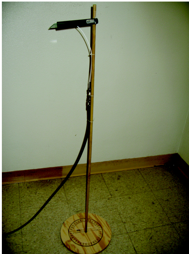
Figure 30-3 Close-up view of PVC antenna mount
