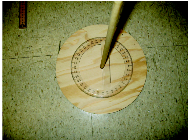
Figure 30-2 View of the circular protractor at the base of the receive antenna
