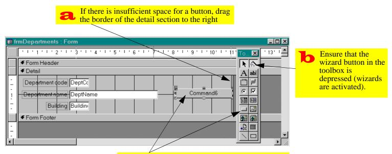
• Select the "command button" tool and click on an appropriate location on the form detail section. The button wizard should appear
