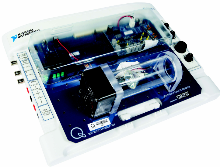
Figure 1: QNET HVAC trainer on ELVIS II.
