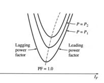
Therefore, by controlling the field current of a synchronous motor, the reactive power consumed or supplied to the power system can be controlled.
