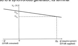
When a generator is operating alone supplying the load:
