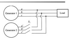
If voltages are not exactly the same in both lines (i.e. in *a* and *a*', *b* and *b*' etc.), a very large current will flow when the switch is closed. Therefore, to avoid this, voltages coming from both generators must be exactly the same. Therefore, the following conditions must be met:
