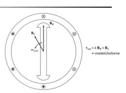
Two magnetic fields are present in the machine, and the rotor field tends to align with the stator magnetic field. Since the stator magnetic field is rotating, the rotor magnetic field will try to catch up pulling the rotor.
