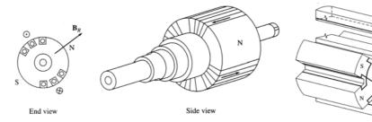
Non-salient-pole rotor: usually two- and four-pole rotors.
