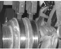
Slip rings are metal rings completely encircling the shaft of a machine but insulated from it. One end of a DC rotor winding is connected to each of the two slip rings on the machine's shaft. Graphite-like carbon brushes connected to DC terminals ride on each slip ring supplying DC voltage to field windings regardless the position or speed of the rotor.
