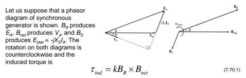
clockwise, opposing the direction of rotation. In other words, the induced torque in generators is a counter-torque that opposes the rotation caused by external torque.
