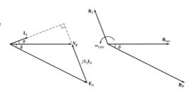
At this point, the machine operates at steady state and synchronous speed but as a motor.
