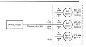
Let us consider a large power system operating at 480 V. Load 1 is an induction motor consuming 100 kW at 0.78 PF lagging, and load 2 is an induction motor consuming 200 kW at 0.8 PF lagging. Load 3 is a synchronous motor whose real power consumption is 150 kW.
