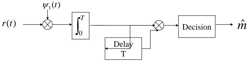
Sub-optimum differentially coherent detector
