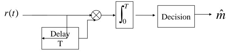
Performance degradation about 3 dB by using suboptimal detector
