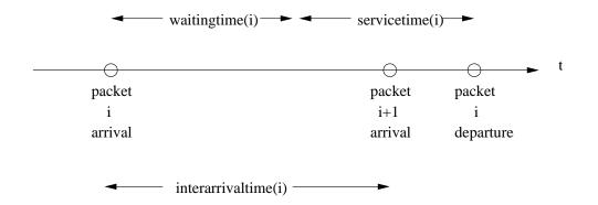
Continuing in this way, we can simulate the arrival time, service time, waiting time, and departure time of each message packet. Using the preceding figure, one can show that the waiting times are generated recursively by the following equation in Matlab syntax:
