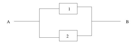
Run the following Matlab script, which estimates the expected lifetime of the relay circuit.
