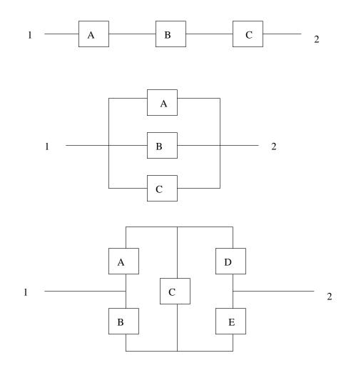
**Problem 6.2:** In each of the three relay circuits above, the switches  $A, B, C, \ldots$  are 90% reliable and work independently. In each case, compute the probability that the relay circuit will relay a signal from point 1 to point 2.
