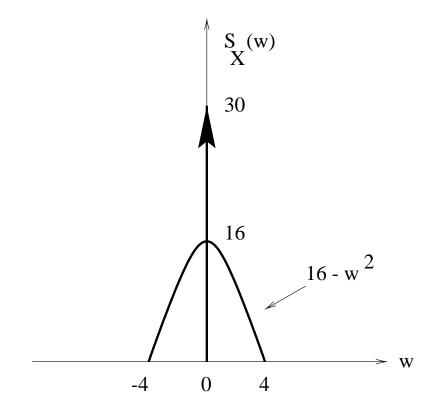
**Problem 3.5:** The power spectral density  $S_X(\omega)$  of an ergodic WSS process X(t) is plotted above.
