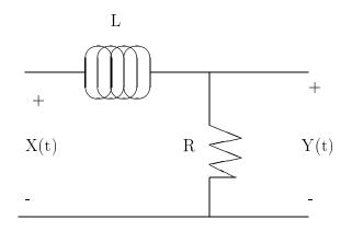
**Problem 4.6:** The input X(t) to the filter above is WSS with autocorrelation function
