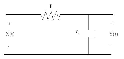
**Problem 4.4:** Refer to the RC filter diagram above. Suppose that RC = 2.
