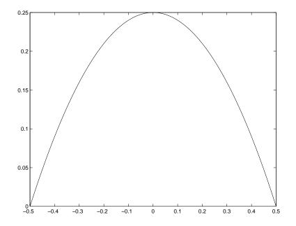
The signal is clearly nonnegative and even. The peak value (which is 0.25) is taken on when t = 0. Half the peak value (which is 0.125) is taken on at  $t = \pm 1/\sqrt{8} = \pm 0.3536$ .
