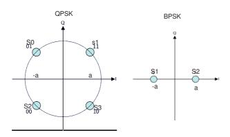
Figure 7.1. QPSK and BPSK modulations
