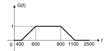
To implement this algorithm, we need to specify two vectors, one containing six frequencies each normalized to Nyquist frequency, the other containing the desired amplitude response at the six specified frequencies. Lastly, we apply the **remez** command to derive the filter coefficients. The order of the filter is taken to be the number of coefficients less one.
