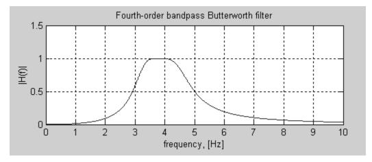
The signal processing toolbox offers more straightforward command for the design of analog filters.
