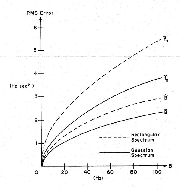
FIG. 6 Normalized RMS Error Versus True Bandwidth
