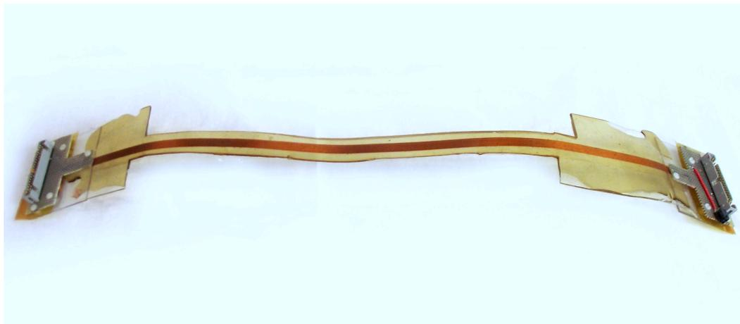
Figure 4.2: Initial prototype for a drive construct where the drive is made of a single conductor that wraps around the entire circumference of the pipeline. This design was intended to reduce the footprint demonstrated by the sensor pictured in Figure 3.4, but actually had the opposite effect.
