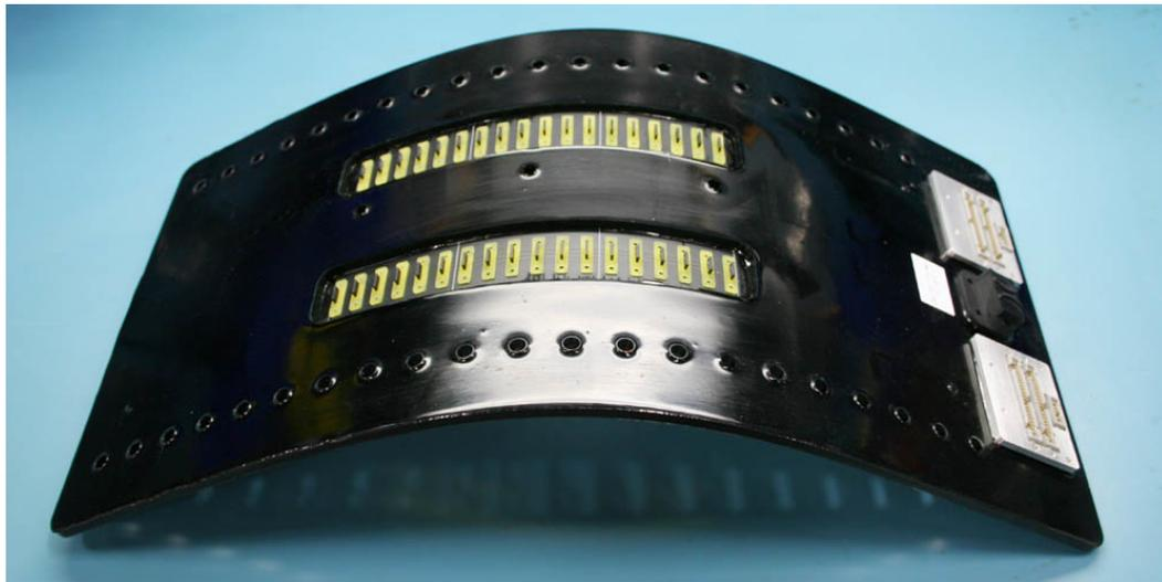
Figure 4.12: The flexible, double row, double rectangle MR-MWM-Array.
