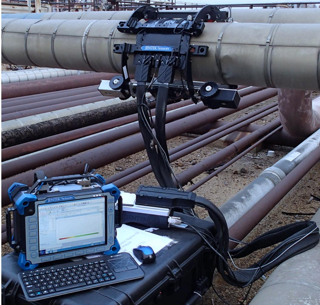
Figure 6.1: Full CUI system including MR-MWM-Array sensor, scanner and instrumentation electronics in the field during performance trials.
