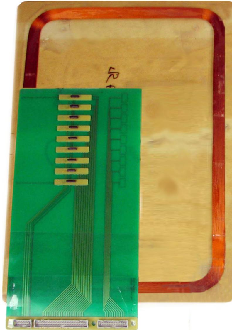
Figure 2.12: Magneto-resistive sense elements spaced 0.5" apart mounted on flexible FR4, which is suitable for wrapping around curved surfaces. Strain relief boards are in-line with the MR chips and decoupling capacitors to allow for achieving a 2" curvature radius without damaging the electronics. The MR-MWM-Array is mounted onto a wound drive with 80 turns of 26 gage rectangular wire.
