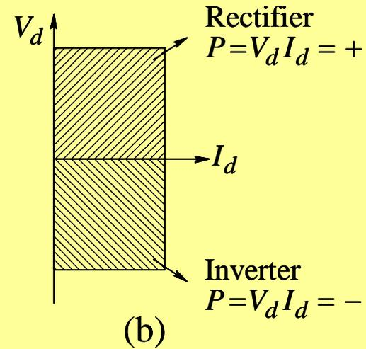
$$V_d = \frac{1}{\pi} \int_{\alpha}^{\alpha+\pi} \hat{V}_s \sin \omega t \cdot d(\omega t) = \frac{2}{\pi} \hat{V}_s \cos \alpha$$
