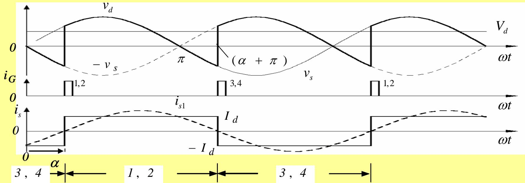
$$v_d(t) = v_s(t) \quad \text{and} \quad i_s(t) = I_d \quad \alpha < \omega t \leq \alpha + \pi$$
