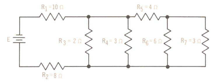
• Redraw the circuit to show series and parallel elements clearly.
