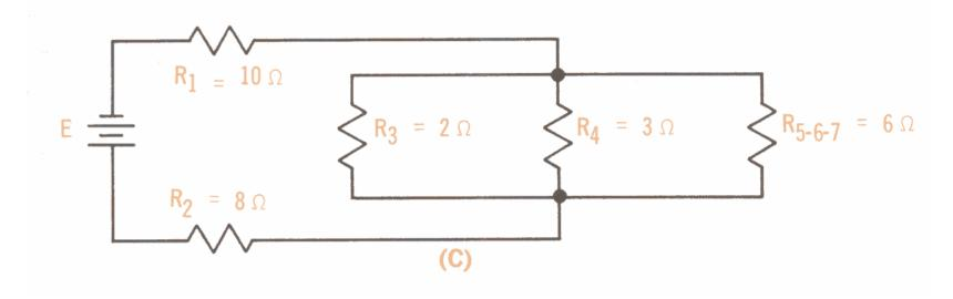
• Replacing R<sub>3</sub>, R<sub>3</sub> and R<sub>5-6-7</sub> (parallel) with their equivalent resistance (1 Ohm) yields a simple series circuit which simplifies by adding and we're done.
