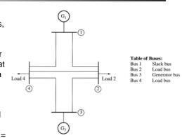
0.3 pu,  $Q_2 = 0.2$  pu,  $P_4 = 0.2$  pu,  $Q_4 = 0.15$  pu (powers supplied to the system at each busses are negative of the above values). The series impedances of each bus were evaluated in Example 11.1. Determine voltages at each bus for the specified load conditions.
