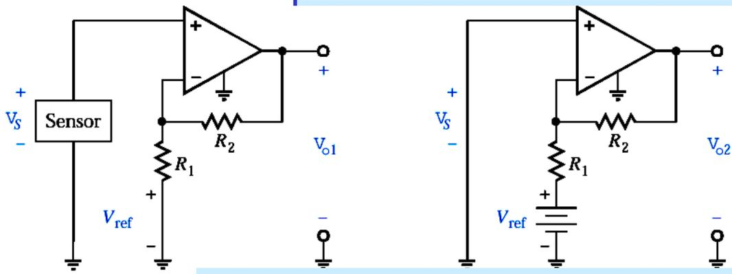
Analyzing circuit using superposition
