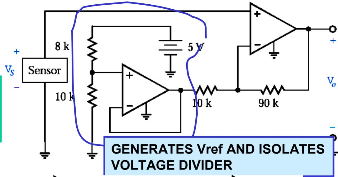
GENERATES  $V_{ref}$  AND ISOLATES VOLTAGE DIVIDER
