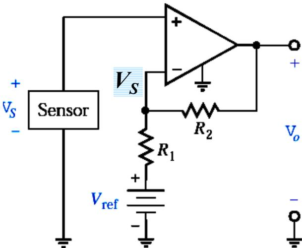
$$0 = \left[ 1 + \frac{R_2}{R_1} \right] (0.5) - \frac{R_2}{R_1} V_{ref} \Rightarrow \frac{R_1}{R_2} = 9$$
