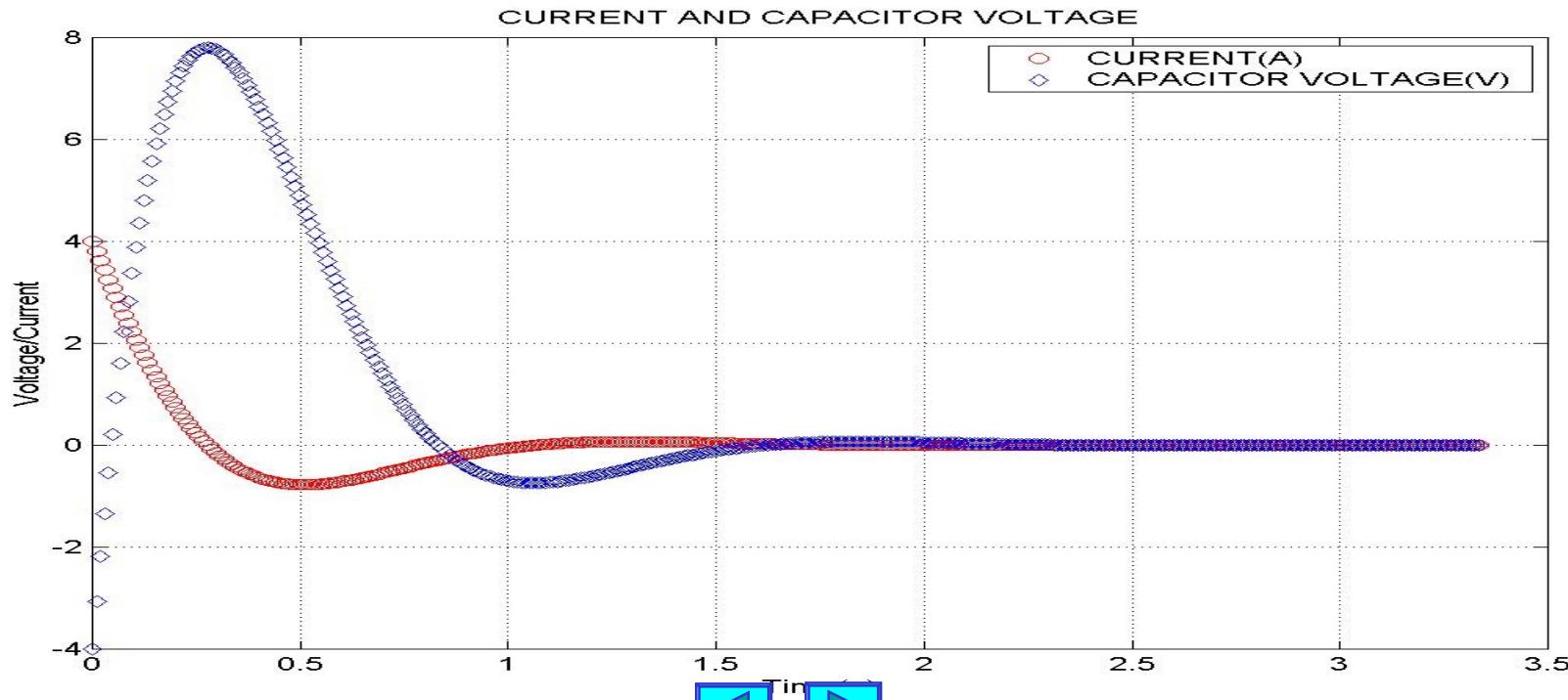
**LEARNING EXAMPLE**  $R_1 = 10\Omega$ ,  $R_2 = 8\Omega$ ,  $C = 1F$ ,  $L = 2H$   $v_C(0) = 1V$ ,  $i_L(0) = 0.5A$
