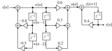
The second-order section can be seen to be cascade of two sections. Interchanging their ordering we finally arrive at the structure shown below:
