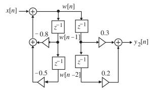
Interchanging the order of the two sections we arrive at an equivalent structure shown below:
