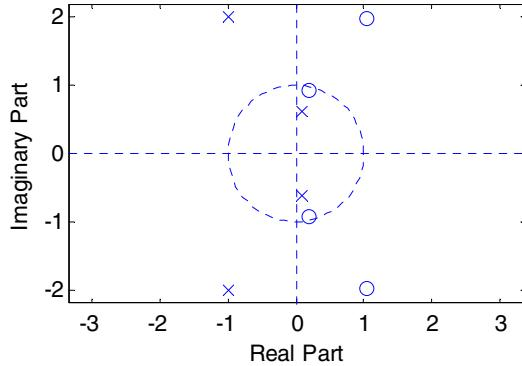
There are 3 ROCs associated with  $G_1(z)$ :  $\mathcal{R}_1 : |z| < \sqrt{0.4}$ ,  $\mathcal{R}_2 : \sqrt{0.4} < |z| < \sqrt{5}$ , and  $\mathcal{R}_3 : |z| > \sqrt{5}$ . The inverse  $z$ -transform corresponding to the ROC  $\mathcal{R}_1$  is a left-sided sequence, the inverse  $z$ -transform corresponding to the ROC  $\mathcal{R}_2$  is a two-sided sequence, and the inverse  $z$ -transform corresponding to the ROC  $\mathcal{R}_3$  is a right-sided sequence.
