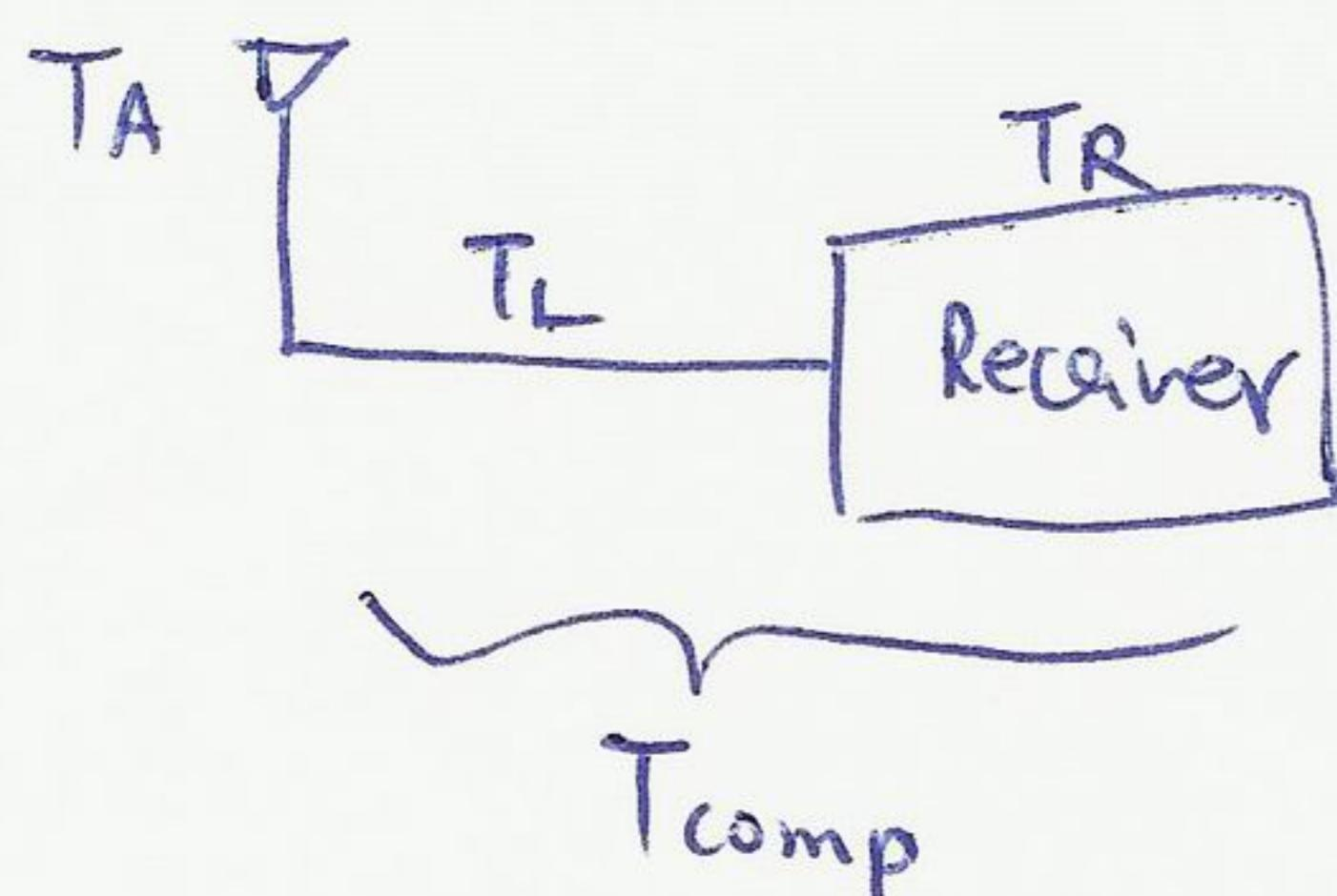
$$\begin{aligned} T_s &= T_A + T_{\text{comp}} \\ &= T_A + T_L + L T_R \\ &= T_A + (L-1) T_0 + L(F-1) T_0 \\ &= T_A + (LF-1) T_0 \end{aligned}$$
