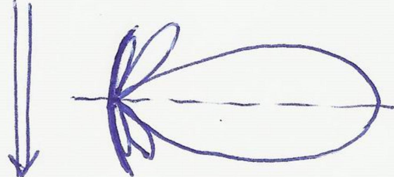
$$p(d) = \frac{P_T G_T}{4\pi d^2} \quad \text{← antenna gain}$$
