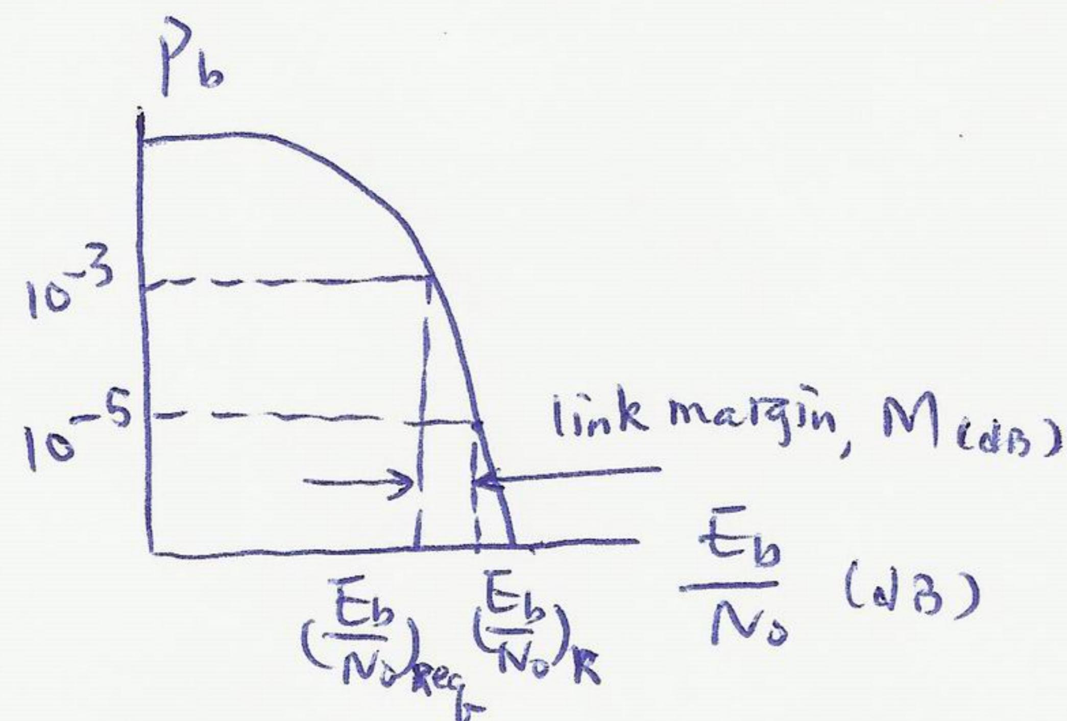
$$\text{Link margin } M_{(\text{dB})} = (\frac{E_b}{N_0})_R (\text{dB}) - (\frac{E_b}{N_0})_{\text{req}_f} (\text{dB})$$
