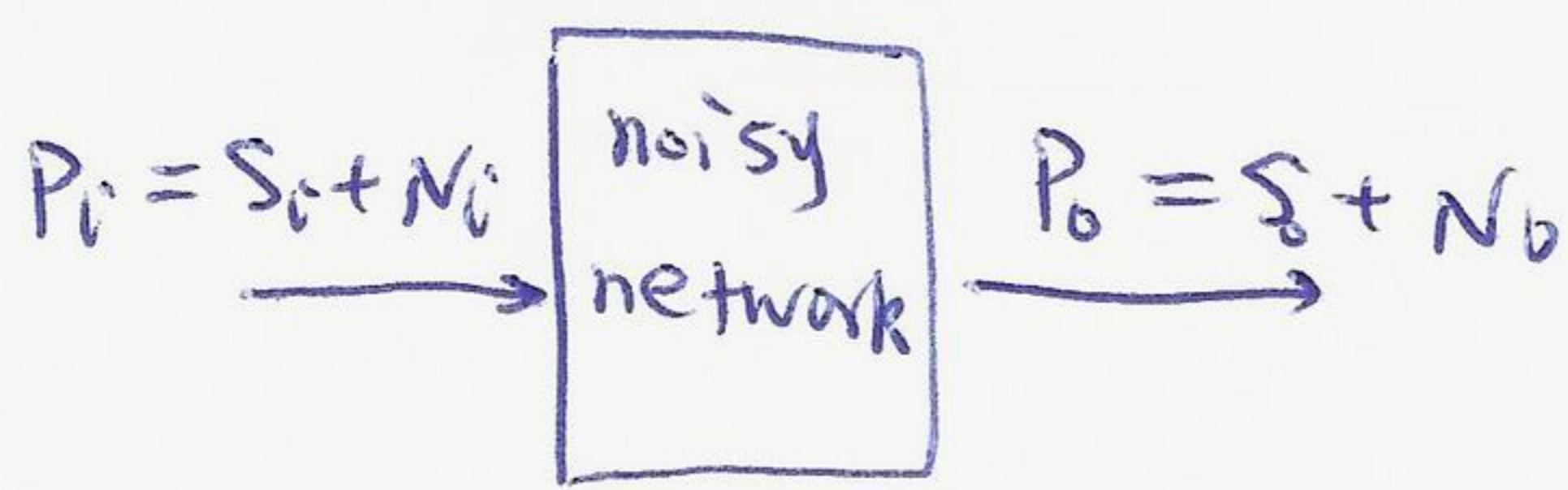
$$F = \frac{(\text{SNR})_{\text{in}}}{(\text{SNR})_{\text{out}}} = \frac{S_i / N_i}{G S_i / G (N_i + N_{ai})}$$
