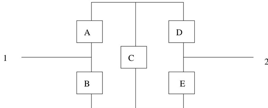
**Problem 6.2:** In each of the three relay circuits above, the switches  $A, B, C, \dots$  are 90% reliable and work independently. In each case, compute the probability that the relay circuit will relay a signal from point 1 to point 2.
