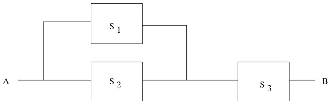
**Problem 6.1:** Consider the relay circuit above for transferring a signal from point A to point B. The components  $S_1, S_2, S_3$  are switches which operate independently of each other. Each switch has only two possible states, “on” or “off”. Let  $p$  be the probability that switch  $S_i$  is on (the same for all three switches).
