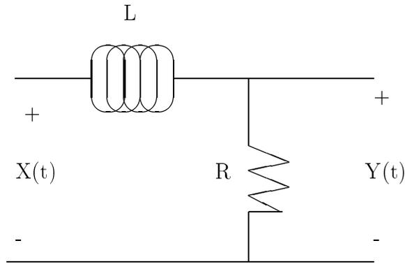
**Problem 4.6:** The input  $X(t)$  to the filter above is WSS with autocorrelation function
