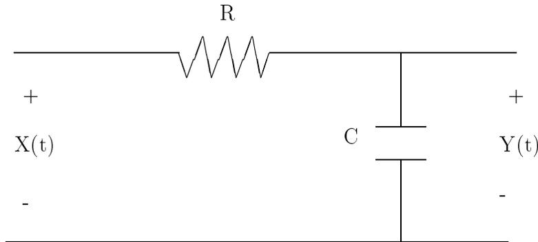
**Problem 4.4:** Refer to the RC filter diagram above. Suppose that  $RC = 2$ .
