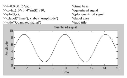
In digital communication, the data format is typically limited by the number of binary digits (bits). Common computer hardware utilizes 8 or 16 bits in the signal value representation. For example, a signal restricted to 8-bit format could consist of a sequence of integers lying between -256 and +255. MATLAB for constructing a single cycle of an 8-bit sinusoide at full amplitude scale might proceed as follows:
