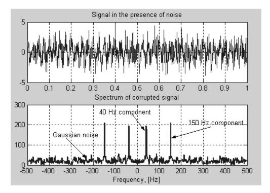
Obviously, it is difficult to identify the frequency components by looking at the original signal in the time domain. On the other hand, the identification of the spectral components is straightforward in the frequency domain.
