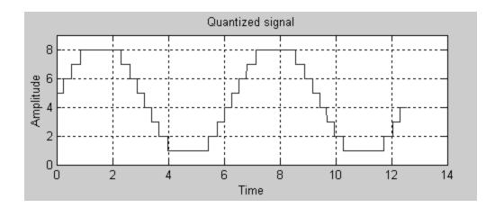
It is possible to adjust the quantization step size by pre-scaling and post-scaling the function values. The following yields functional values limited to one digit to the right of the decimal point.
